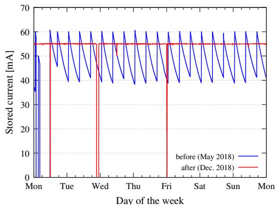
Figure 4: Stored currents of the PF-AR before and after introducing the top-up injection. The current is maintained at  $55 \pm 0.1$  mA after the introduction, while it is topped up three times a day to 60 mA before. The current drops in the figure are due to beam dumps caused by machine issues or re-injections for recovering the sudden drop of the beam lifetime.
