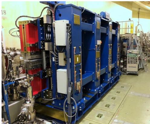
Figure 2: New APPLE-II type undulator installed for the BL19.
