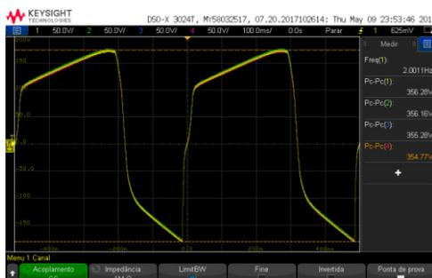
Figure 5: Module output voltages during a ramp (50V/div).
