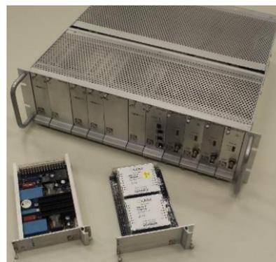
Figure 2: FBP PS, power module and DCCT board.
