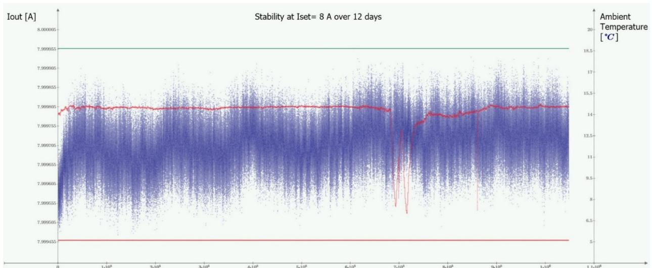
Figure 7: output current stability test over 12 days, along with the ambient temperature recording. The current (the “blue cloud”) remains within 0.5 mA<sub>pk-pk</sub>, corresponding to 30 ppm<sub>pk-pk</sub> referred to nominal output current (16 A).
