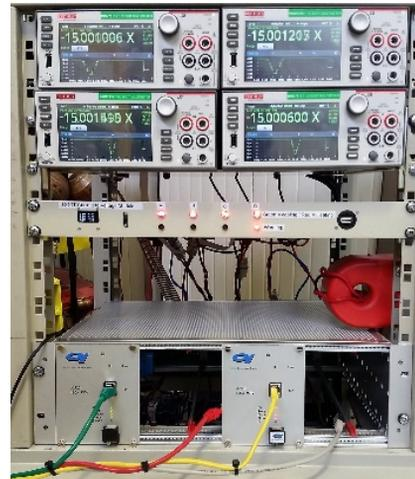
Figure 6: Two pre-series A2720 channels (in their sub-rack) under test in the specifically prepared rack.
