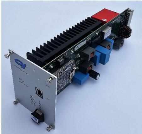
Figure 5: One A2720 channel, on the rear of the card it is visible the large heatsink cooling the H-Bridge.
