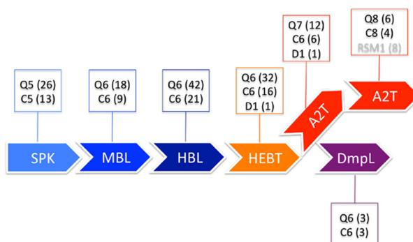
Figure 2: SC structure of the linac with magnet types.
