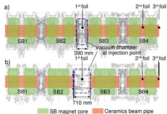
Figure 2: System configuration of the beam injection area. a) Current configuration. b) New configuration under designing for the radiation shield installation.
