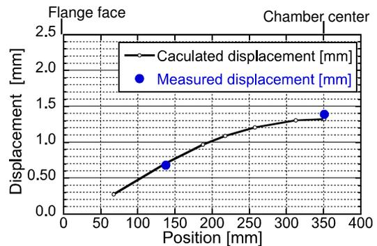
Figure 5: Calculated and measured displacement by the atmospheric pressure of the vacuum chamber.
