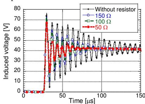
Figure 6: Dependence of the induced voltage modulation on the damping resistor value. The flat top excitation current was 9.5 kA .
