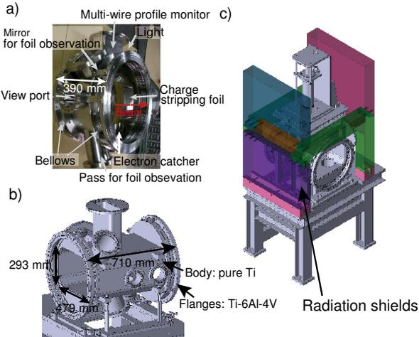
Figure 3: a) Current vacuum chamber at the beam injection point. b) Newly designed vacuum chamber. c) Radiation shield under designing.
