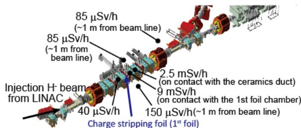
Figure 1: Typical residual dose distribution at the beam injection area in the RCS about 5 hours after beam operation with 500 kW power.
