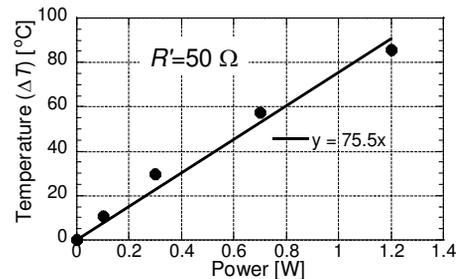
Figure 8: Relation of the temperature rise and power consumption of the 50  $\Omega$  resistor. The dots are measured value and the line is the linear fit.
