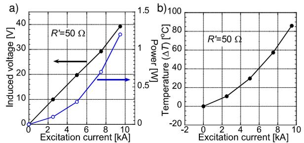
Figure 7: a) Dependence of the voltage and power of a dumping resistor on the excitation current. b) Dependence of the damping resistor temperature on the excitation current.
