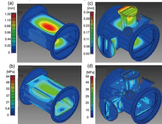
Figure 4: a), b) Calculated displacement and Von Mises stress in a vacuum chamber without bellows and ports. c), d) Those in the vacuum chamber with the final design.
