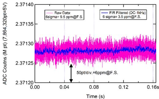
Figure 3: Waveforms of sampled raw data (pink) with 100 kHz, and filtered data (blue) with DC-1kHz in off-line analysis.
