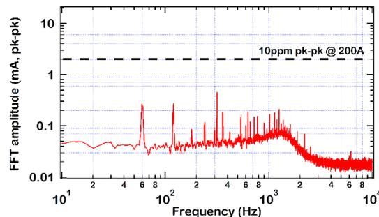
Figure 5: FFT amplitude of output current at 200 A operation.
