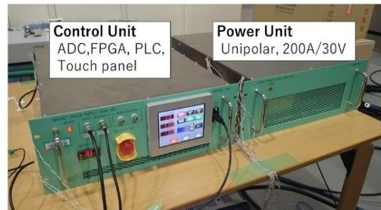
Figure 4: Overview of test PS using the digital feedback control system.
