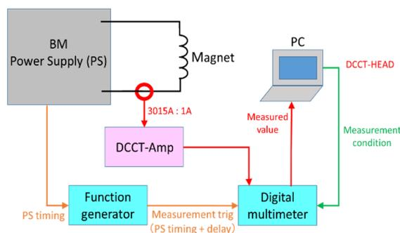
Figure 1: Configuration of the measurement system.
