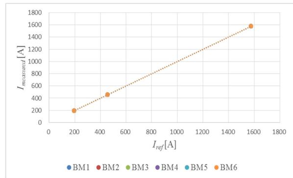
Figure 4: Linearity of reference current and measured current.
