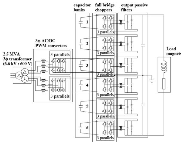
Figure 1: Schematic view of power converter for the bending magnet family in J-PARC MR.
