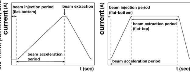
Figure 4: Schematic view of output current pattern in FX (left) and SX (right) mode.
