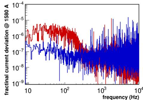
Figure 7: Spectrums of the fractional current deviation in the new BMPS and the present BMPS (red).
