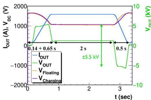
Figure 5: Measured output current, voltage and voltages in charging and floating capacitor in the test with the SX pattern.
