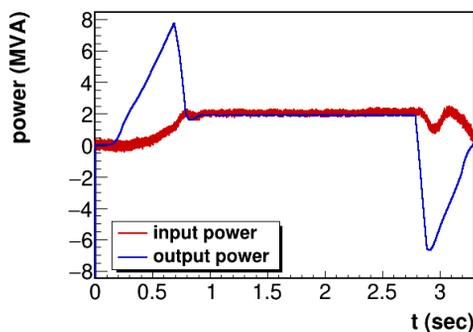
Figure 6: Measured input and output power.
