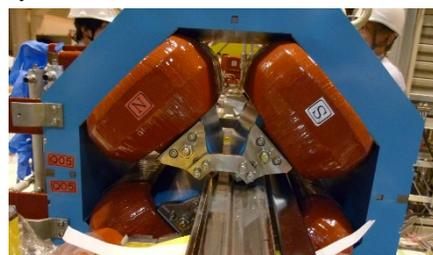
Figure 4: Aligned 12-m LIC and a reassembled quadrupole magnet.
