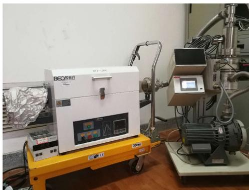
Figure 2: Quantitative deposition coating system.
