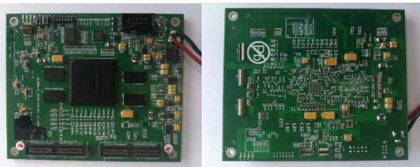
Figure 6: Digital controller motherboard.
