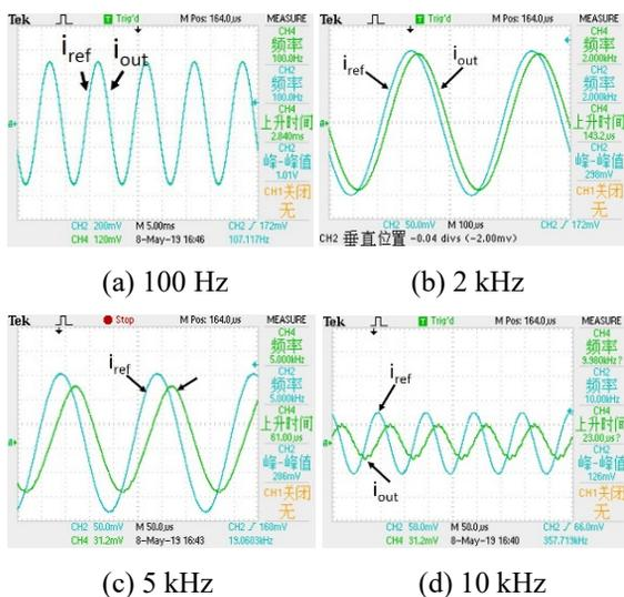
Figure 8: Test curve of bandwidth.
