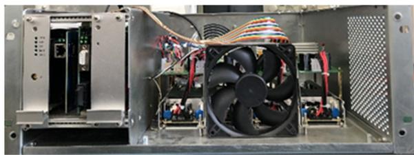
Figure 7: The prototype of power supply.
