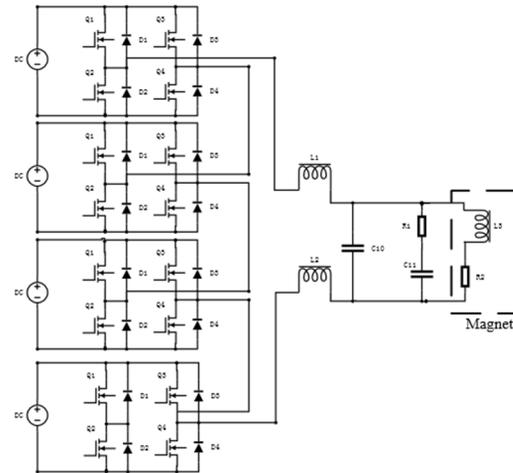
Figure 1: Schematic of power supply.
