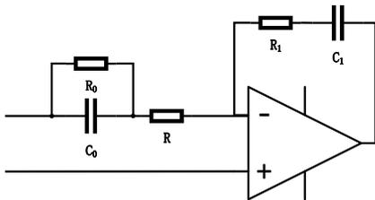
Figure 3: Actual phase-correction design.
