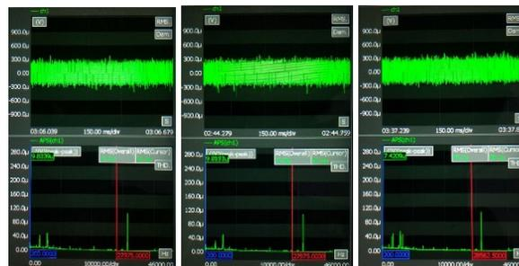
Figure 9: Test curve of output current ripple.
