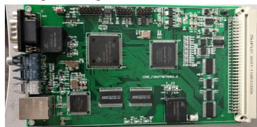
Figure 4: The digital control card.
