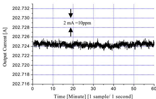
Figure 7: Measured output current stability using a single ADC chip of 16-bit.
