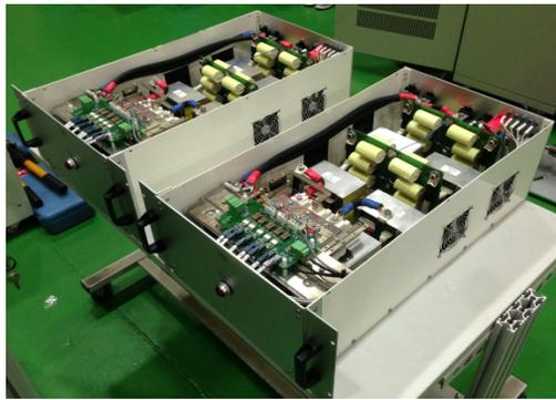
Figure 5: Power converter modules.
