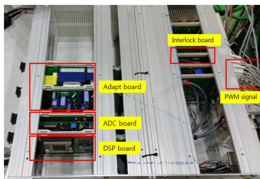
Figure 2: Control board diagram of the MPS.
