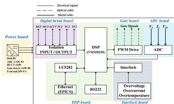
Figure 1: Configuration of the control system.
