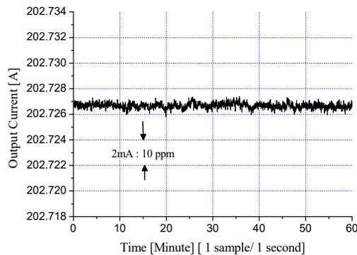
Figure 6: Measured output current stability using a proposed ADC scheme.
