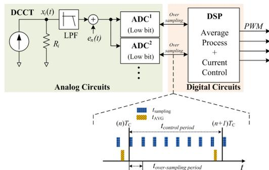
Figure 3: Proposed ADC Scheme and oversampling timing diagram.
