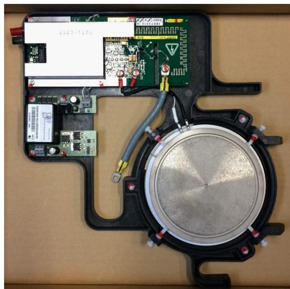
Figure 1 : View of an isolated IGBT module.
