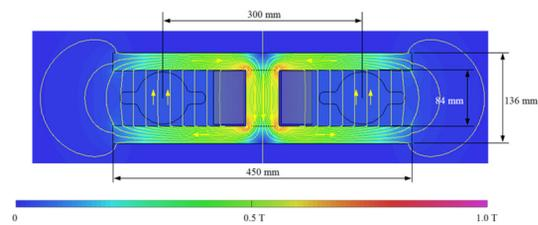
Figure 2: Cross section of the common-yoke dipole [9], with stylized VC cross-sections.
