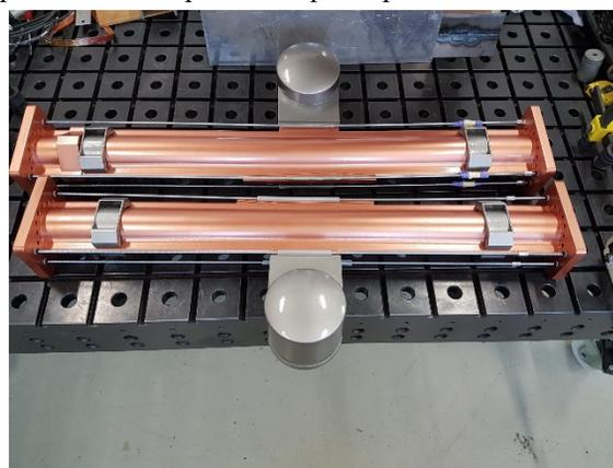
Figure 5: Short prototypes with pumping domes, Matsuoto-Ohtsuka-type flanges, and dummy BPM block.
