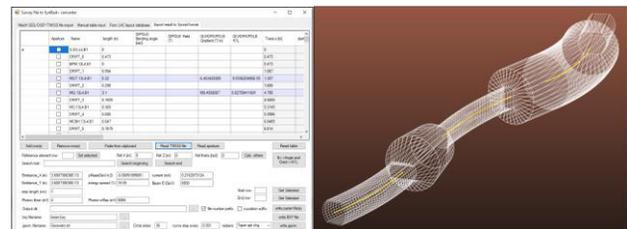
Figure 2: OpticsBuilder interface (left) and generated geometry (right).
