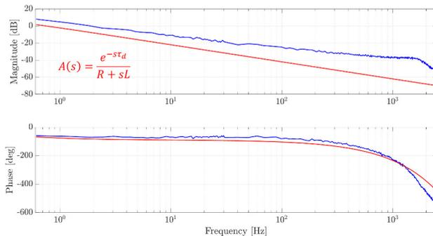
Figure 3: Frequency response of the *trans-admittance* from the power converter reference voltage to the measured current in the magnet. Measured (blue); *nominal* R-L series model including an estimated *digital* delay  $\tau_d \approx 400 \mu\text{s}$  (red).
