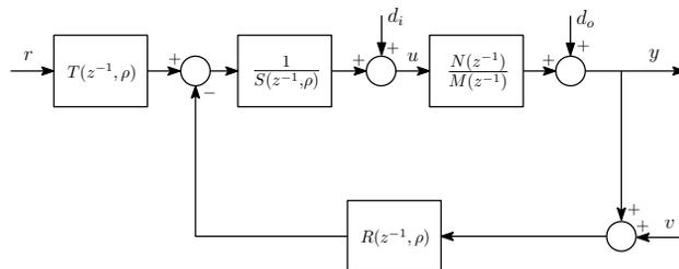
Figure 1: RST controller structure.
