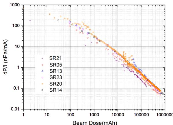
Figure 2: Beam cleaning process for six new vacuum sections.
