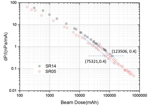
Figure 3: Comparison of  $dP/I$  with different pumping speeds.
