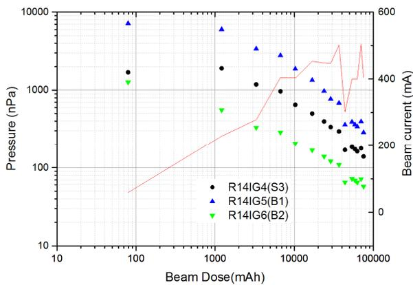
Figure 5: Pressure evolution during beam commissioning in section SR14.
