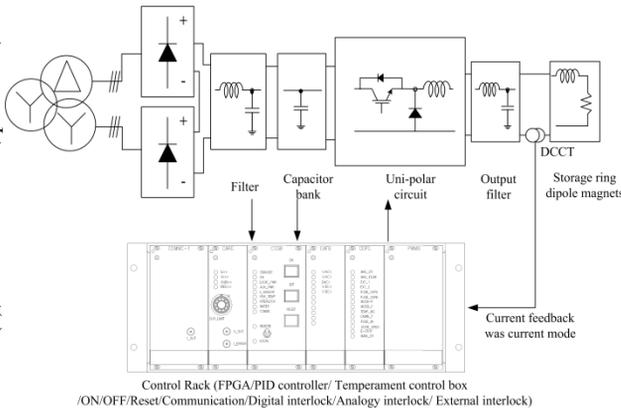
Figure 3: The technology circuit diagram of the bending magnet power converters.
