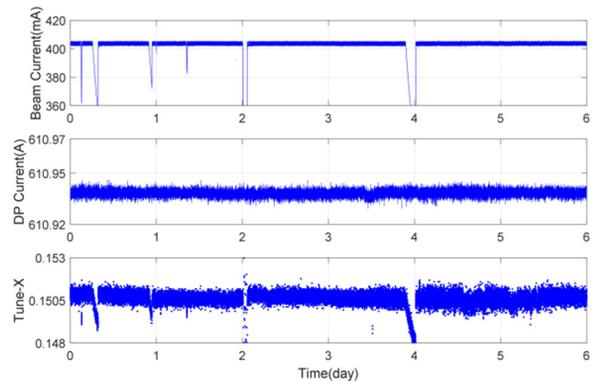
Figure 10: The beam particle position, bending magnet current, and tune-X relationship with adjusting the temperature setting.
