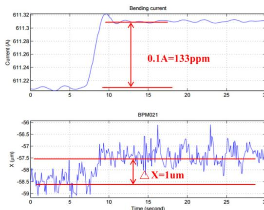
Figure 2: Influence of the bending magnet current variation on beam particle position.
