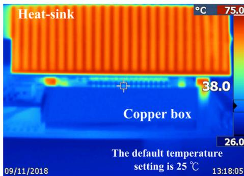
Figure 7: Thermal image of the temperature regulation box with default setting.
