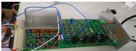
Figure 4: Temperature regulation box of a COMMC card.
