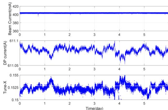
Figure 1: The beam particle position, bending magnet current, and tune-X relationship without adjusting the temperature setting.
