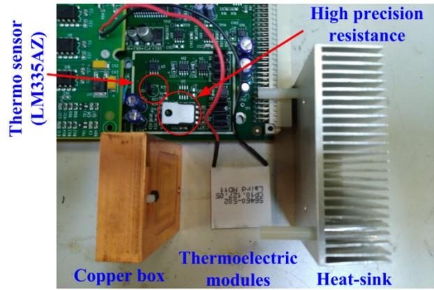
Figure 5: Component of the temperature regulation box.
