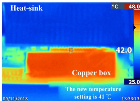
Figure 8: Thermal image of the temperature regulation box with new setting.
