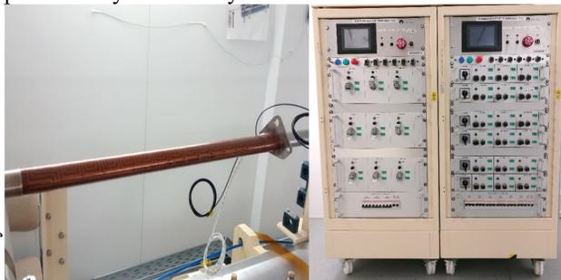
Figure 7: Composite picture showing (left) DDBA vessel wrapped with polyimide bakeout heater and (right) PLC-based bakeout controller developed for DDBA.
