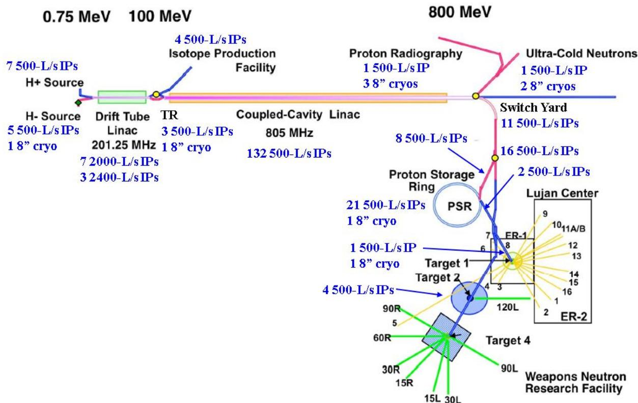
Figure 1: Distribution of ion pumps (IPs) and cryopumps in the LANSCE accelerator complex. (blue letters)
