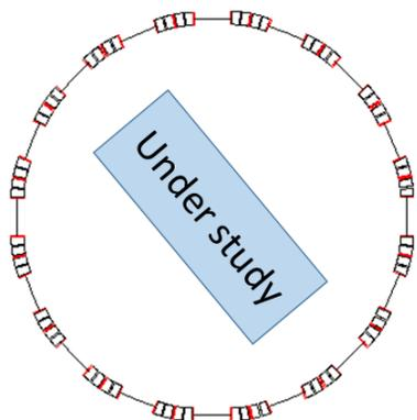
Figure 2: Simplified lattice currently under study with the developed model. This is a proton frozen spin lattice with an energy of  $\approx 230$  MeV. It is composed of 64 electrostatic deflectors + fringe fields with a radius of 32 m and an electric field of  $\approx 13$  MV/m. The focusing is done with magnetic quadrupoles, with no effect on the spin.
