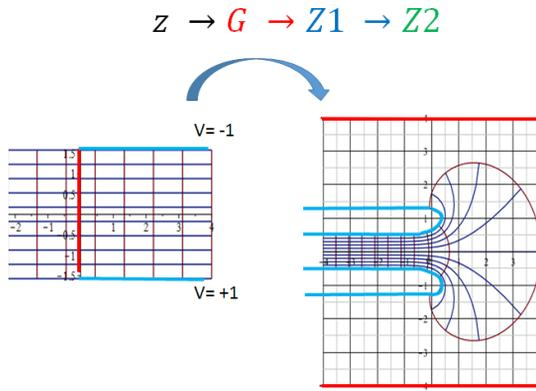
Figure 1: Left : Semi-infinite box with straight electrodes (blue) and zero equipotential boundary condition (red). The potential in this system is known (see [3]). Right : view from above of a realistic deflector with vacuum chamber and diaphragm (red) and curved electrodes (blue). The equipotential and field lines are here for illustration.
