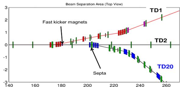
Figure 3: Lattice of the TD20 extraction beam line and the LUXE experiment. The beam line starts with the fast kicker magnets, 4 Lambertson septa magnets bend the beam towards the TD20 tunnel. Courtesy: N. Golubeva.
