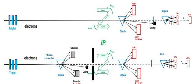
Figure 1: Experimental scenarios for the LUXE experiment. Stage 1 (top): electron bunch — laser collision, stage 2 (bottom): photon — laser collision with the photoconverter foil upstream of the Interaction Point.
