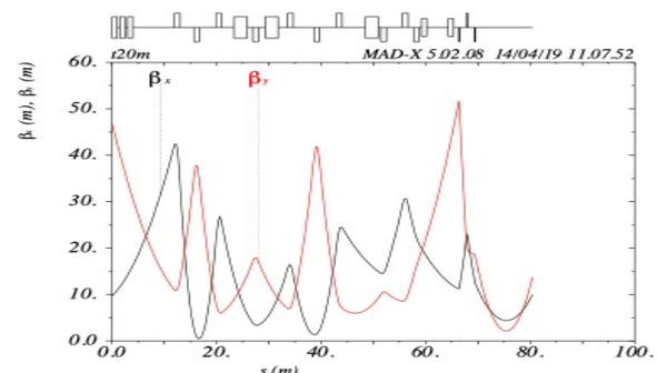
Figure 4: Beam optics simulation with MADX downstream of the septa and final focus to the experiment.
