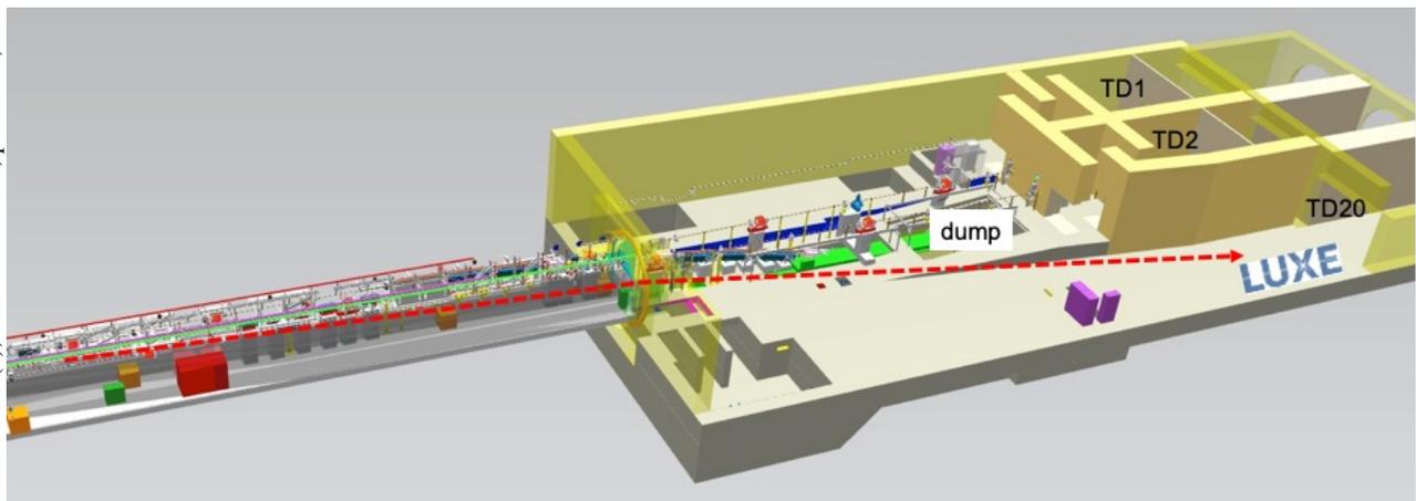
Figure 5: CAD model of the end of the European XFEL accelerator tunnel and the shaft building with the two existing beamlines T1 and T2 to the undulators and the TD20 tunnel, where the LUXE experiment will be installed. The beam extraction and the beam line towards the experiment is sketched with the dashed line.
