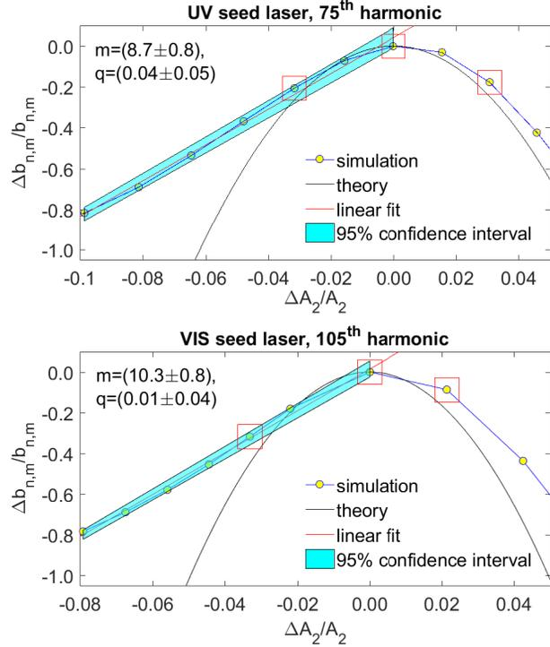
Figure 3: Comparison of relative bunching deviation as a function of the relative deviation in  $A_2$  factor between vis and uv seed laser. The red boxes indicated the simulation points selected for Fig. 4.
