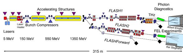
Figure 1: Layout for the FLASH 2020+ upgrade.
