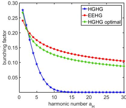
Figure 2: Bunching factor as a function of the harmonic number. The red dots represent the maximum of EEHG bunching factor for the considered working point (Tab. 1). The blue dots are the HGHG bunching factor calculated using the optimal parameters ( $A_2$  and  $B_2$ ) for the EEHG. Finally the yellow dots represent the HGHG bunching with optimized parameters.
