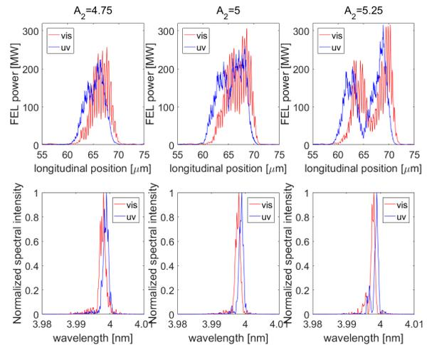
Figure 4: Performance of FEL power as seed laser power is changed for both uv and vis seed lasers.
