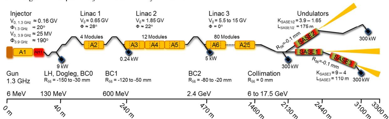
Figure 1: Schematic overview of the European XFEL accelerator, switch yard and undulator beam lines.
