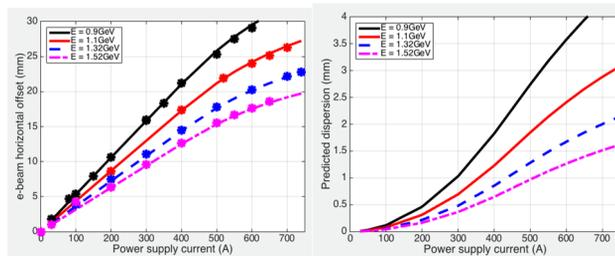
Figure 7: Left) Electron beam offset measurements compared to theoretical predictions. Right) prediction for induced dispersion.
