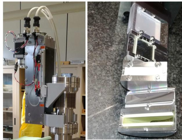
Figure 4: Left) Vacuum manipulator used for inserting on axis the seed laser mirror and the photon/electron diagnostic. Right) Vacuum components installed on the manipulator.
