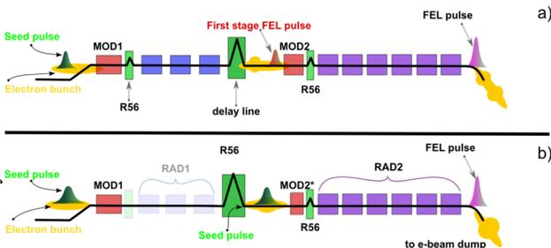
Figure 1: a) Nominal layout of FEL-2 for HGHG-FB. b) Modified layout used for the EEHG experiment.
