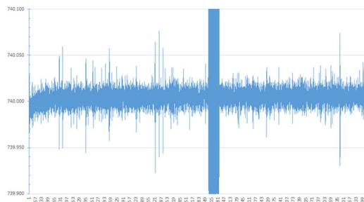
Figure 3: Stability of the power supply current at 750A with the configuration used for EEHG experiment.
