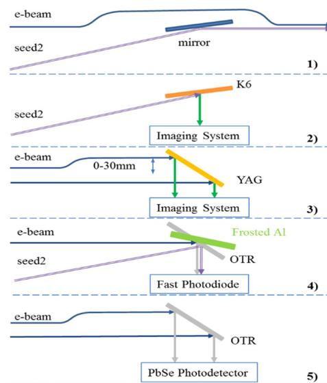
Figure 5: Diagnostic configuration.
