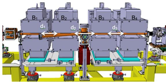
Figure 2: Drawing of the delay-line chicane.
