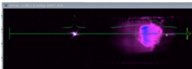
Figure 6: e-beam position (bright spot) measured with the YAG screen. Signal detected on the right side comes from CSR signal produced by the beam when passing through the magnets.
