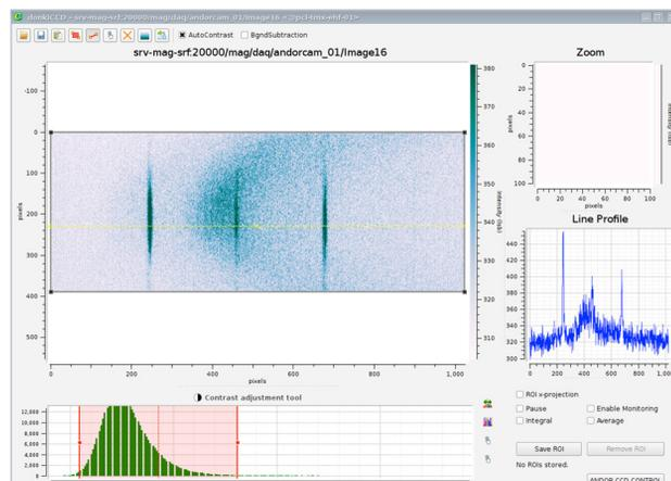
Figure 8: Central peak refer to the second diffraction order of the radiation at harmonic 101. Lateral peaks refer to first diffraction order of the radiation emitted at harmonics 50 and 51.
