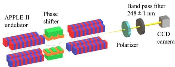
Figure 2: Schematic illustration of the experimental configuration. This figure is reproduced from ref [8].
