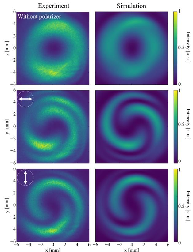
Figure 3: Obtained intensity distributions in experiment (left column) and simulation (right column). Top row shows intensity without polarizer. Middle and bottom rows show intensity through horizontally and vertically oriented polarizer.
