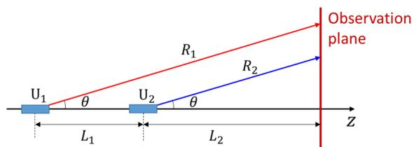
Figure 2: Schematic layout of a simple crossed-undulator configuration.
