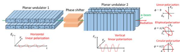
Figure 1: Conceptual configuration of the crossed-undulator.
