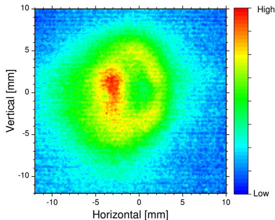
Figure 1: Observed CER profile at KU-FEL. The electron beam moves from the center to the left.
