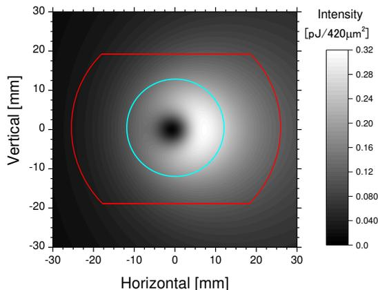
Figure 3: Calculated CER profile at the concave mirror in the FEL optical cavity. The electron beam moves from the center to the right.
