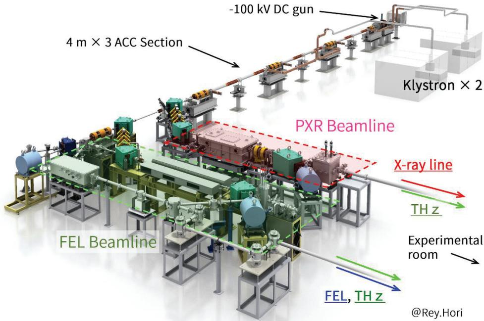
Figure 1: Layout of the 125MeV electron linac at LEBRA in Nihon University. LEBRA-linac consists mainly of the -100 kV electron DC-gun, the pre-buncher, the buncher and the three 4 m long traveling wave accelerating tubes. The main purpose of LEBRA-linac is the generation of FEL, PXR and THz.
