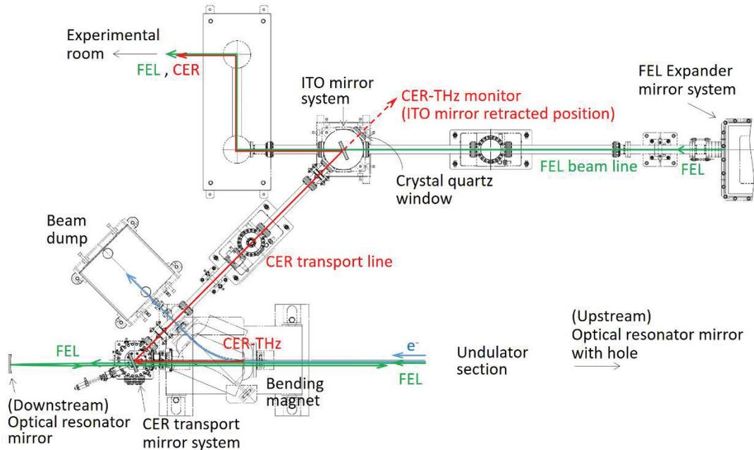
Figure 2: Schematic diagram of the improved CER-THz transport system. A sapphire substrate with a thickness of 0.5 mm sputtered with 400 nm of ITO was placed. ITO substrate can reflect THz waves with a frequency of 1 THz by 80% or more. The crystal quartz vacuum window of the extraction viewport is attached to reduce THz transmission attenuation. The mirrors of the CER transport mirror system were replaced from concave mirrors to toroidal surface mirrors.
