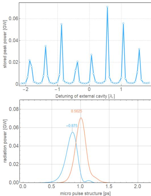
Figure 4: An example of pulse stacking. The detuning scan (upper) is performed at each  $\lambda_r/16$ . Each value displayed in the bottom figure corresponds to the detuning value in the unit of radiation wavelength.
