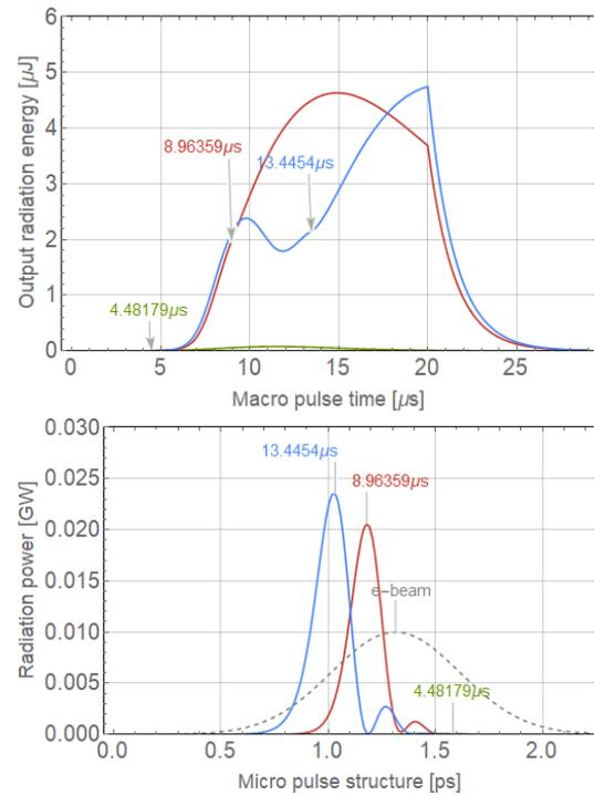
Figure 3: A macro-pulse waveform of accumulation with the dynamical detuning (upper figure), and the corresponding pulse structures (bottom figure). We start from the cavity detuning length  $\Delta L = -0.75 \lambda_r$ , and change to the zero-detuning at each arrow point respectively.
