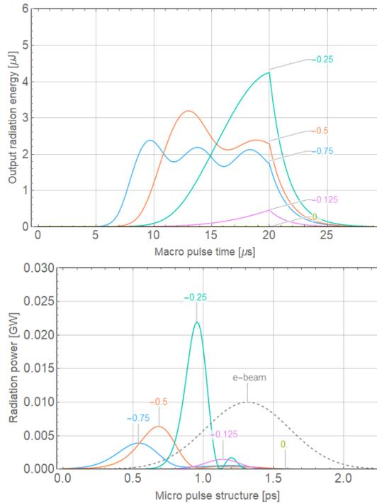
Figure 2: A macro-pulse waveform of accumulation without the dynamical detuning (upper figure), and the corresponding pulse structures (bottom figure). Each number displayed suggests the cavity detuning length in the unit of radiation wavelength  $\lambda_r$  respectively.
