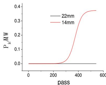
Figure 1: Resonator power as a function of the optical pass to waveguide gap 14mm and 22mm when the radiation frequency is 1THz.
