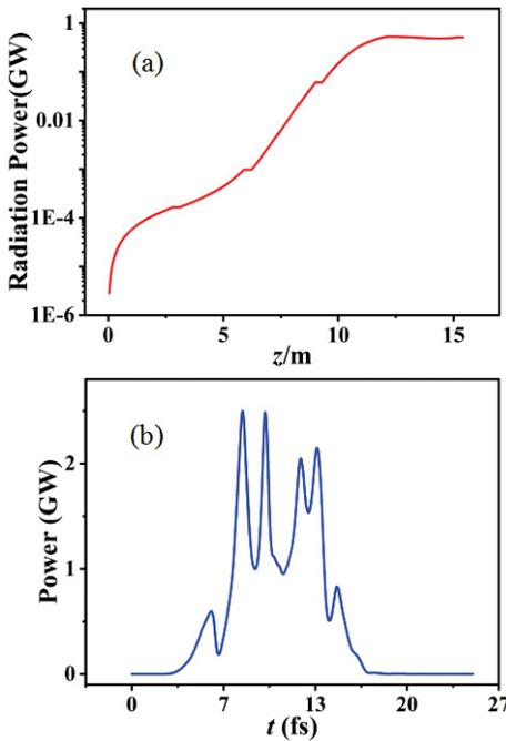
Figure 6: (a) Power gain along undulator line, (b) power temporal profile of radiation pulse at  $z = 12.3$  m.
