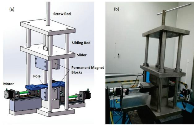
Figure 3: Prototype of PMSU: (a) 3D drawing, (b) physical object
