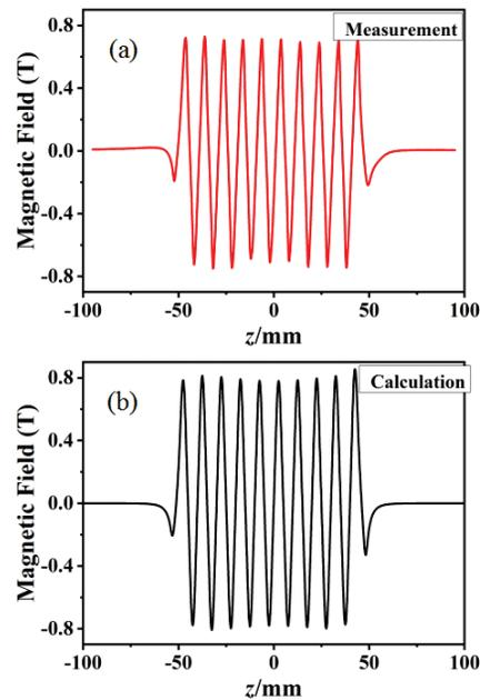
Figure 4: Distribution of periodic field: (a) calculation, (b) measurement
