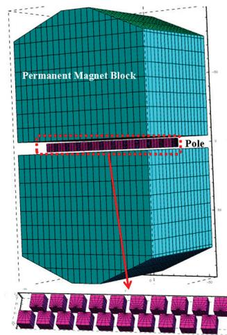
Figure 1: Magnetic structure of PMSU in Radia.
