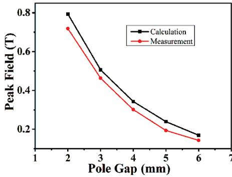
Figure 5: Peak field VS pole gap.
