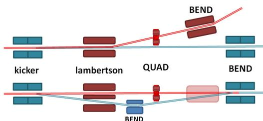
Figure 7: The layout of the beam distribution system.
