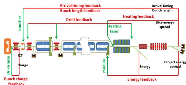
Figure 8: The layout of the injector feedback system.
