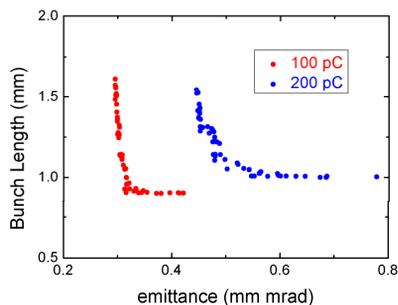
Figure 2: Multi-objective optimization results of the injector.
