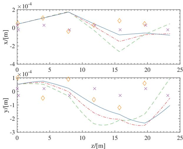
Figure 1: The initial horizontal (up) and vertical (down) quadrupole misalignment (orange-diamond), BPM offsets (purple-cross), electron orbit at 840 MeV (blue), 730 MeV (red), 610 MeV (green).
