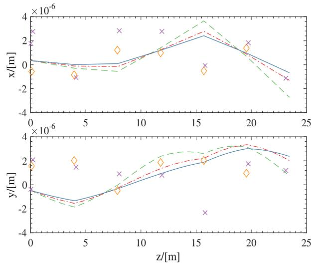
Figure 2: The position of quadrupoles (orange-diamond) and BPMs (purple-cross), the electron beam trajectories at 840 MeV (blue), 730 MeV (red), 610 MeV (green) after correction in the horizontal (up) and vertical (down) planes.
