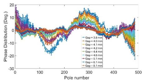
Figure 9: On the top, the RMS phase error as a function of the gap. On the bottom, the phase distribution versus the pole number at different gaps.
