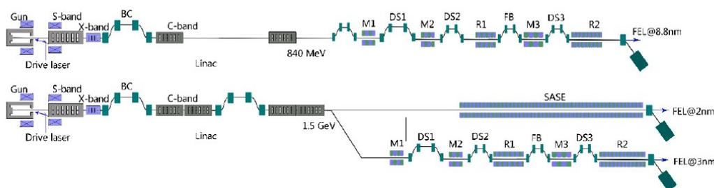
Figure 1: Schematic layouts: SXFEL-TF (upper) and SXFEL-UF (lower)[1].
