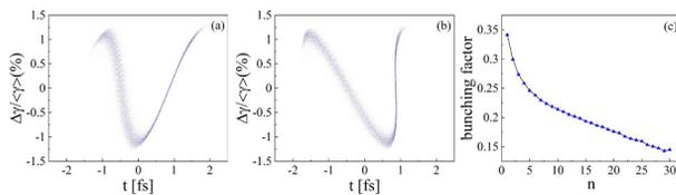
Figure 5: Longitudinal phase space distributions at the exits of the modulator (TGU) (a) and the first dispersion section (C1) (b) and the corresponding bunching factor for  $n_{th}$  harmonic (c). One electron slice ( $= \lambda_s = 800$  nm) has been highlighted to show the principle.
