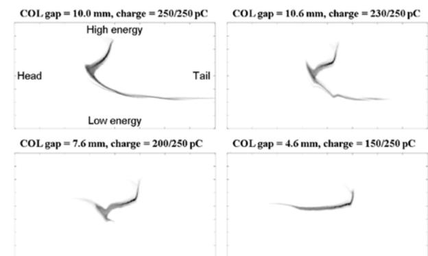
Figure 5: Variation of the longitudinal phase space by the gap of BC1 collimator. These are the results of ELEGANT simulations.
