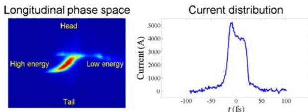
Figure 3: Longitudinal phase space and current distribution of electron bunch at the end of linac section for nominal operation. These results are measured in the BAS3H.
