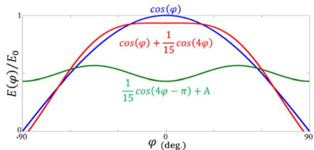
Figure 1: Linearization of the RF electric field curvature with a high harmonic cavity.
