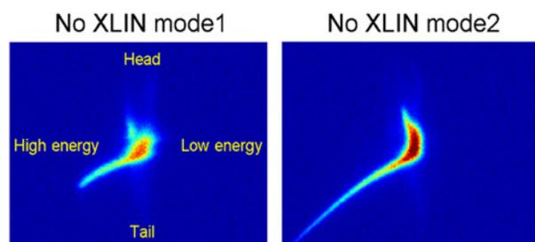
Figure 6: Longitudinal phase spaces of two FEL operation modes without XLIN.
