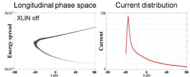
Figure 4: Longitudinal phase space and current distribution of electron bunch at the end of linac section for the operation without XLIN and collimators. These are the results of ELEGANT simulations.
