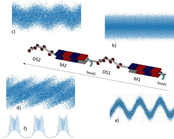
Figure 1: Layout of the EEHG scheme before the radiator with illustrations of how the electron beam phase space looks at each stage. After the first modulator M1 a), after the first dispersive section DS1 b), after the second modulator M2 c), after the second dispersive section DS2 d). Picture f) shows the current profile at the exit of DS2.
