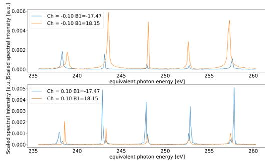
Figure 2: Harmonic content of bunching for positive (top) negative (bottom) chirp having the first dispersive section with different signs. Simulations are optimized for harmonic 52 of a seed laser  $\lambda_{mod1} = 260nm$  for a non chirped beam.
