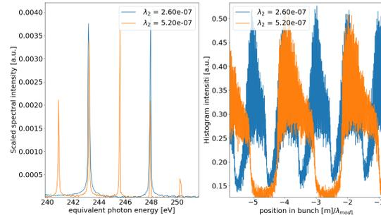
Figure 3: Figure presenting the harmonic content of bunching (left) and beam distribution histogram (right) for two second modulator wavelengths  $\lambda_{mod2} = 260nm$  and  $\lambda_{mod2} = 520nm$ .
