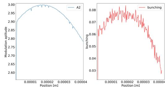
Figure 4: Figure comparing the amplitude modulation (left) after MOD2 to bunching level along the electron pulse at entrance to the radiator (right) of a chirped beam going through the layout in Fig. 1.
