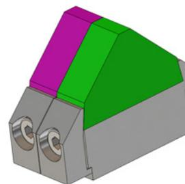
Figure 6: Schematic of magnet module with two magnet blocks.
