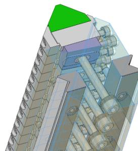
Figure 5: Schematic of undulator sub-girder with wedge and spring loaded magnet module.
