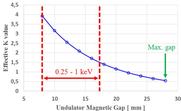
Figure 2: Operational gap range of the APPLE X undulator.
