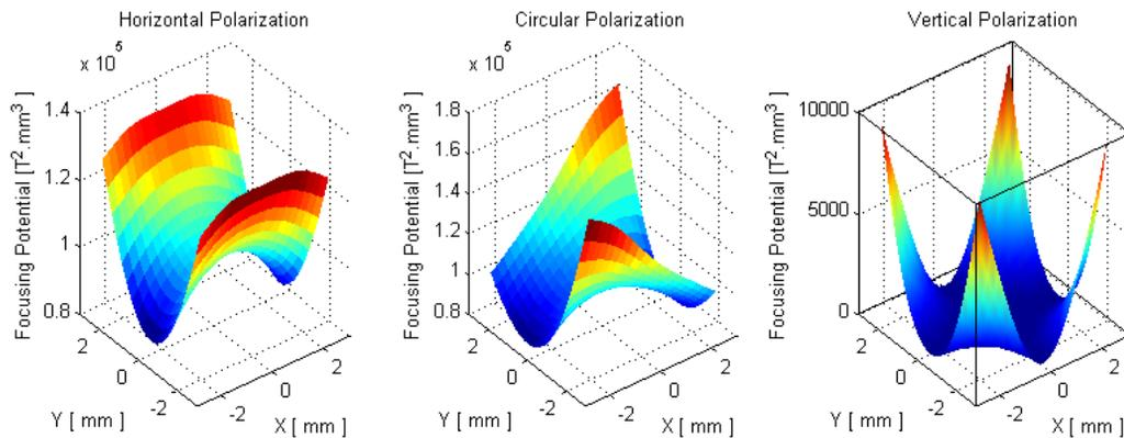
Figure 7: APPLE X undulator focusing potential for horizontal, vertical and circular modes at minimum gap of 8 mm.
