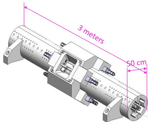
Figure 3: Schematic view of compact APPLE X undulator.
