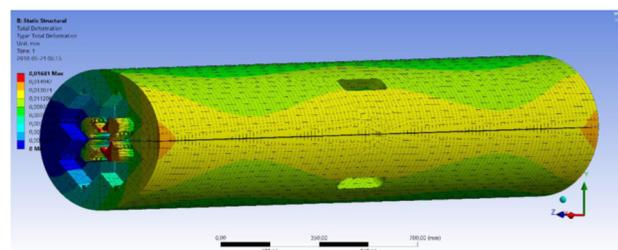
Figure 4: Undulator FEA model gives maximum 7  $\mu\text{m}$  deformation along the bulk and <15  $\mu\text{m}$  at the extremities.
