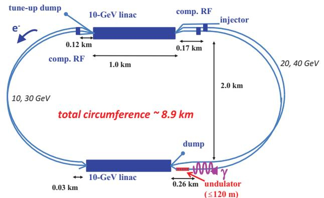
Figure 1: LHeC ERL reconfigured for FEL operation.
