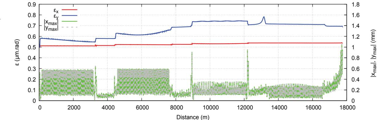
Figure 4: Simulated evolution of the two transverse normalized emittances (after subtracting dispersive contributions) and maximum particle position while decelerating the spent beam over 2 complete LHeC turns from 40 to 0.6 GeV.
