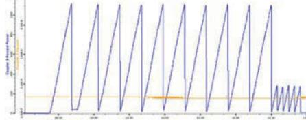
Figure 3: Example of RF power ramps up to 1.1 MW applied during RF conditioning of a coupler pair.
