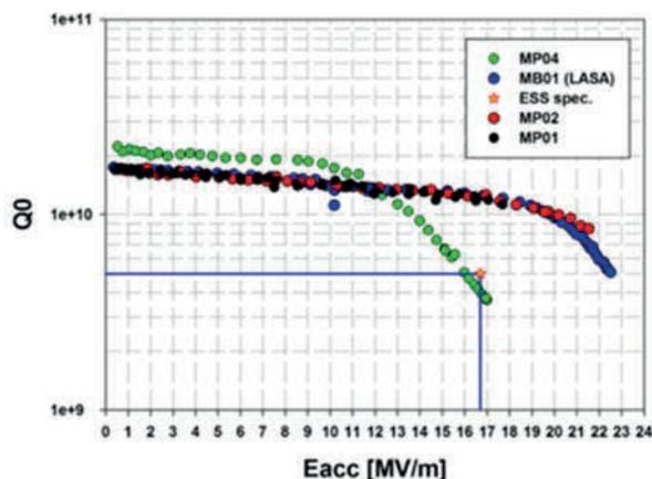
Figure 2: Q curves of the cavities before assembly in the M-ECCTD.
