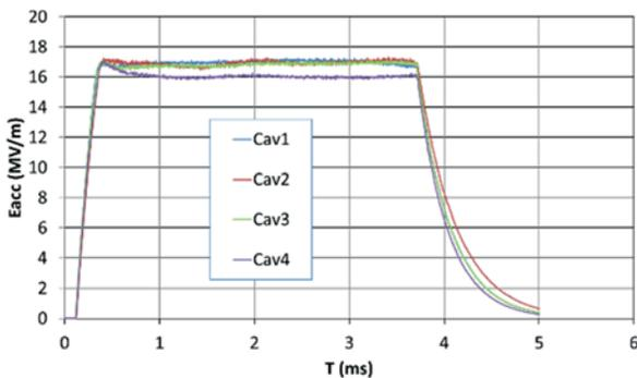
Figure 7: The four cavities pulses with static pre-tuning, piezo compensation and 4P/P klystron output pulse.
