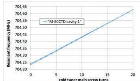
Figure 5: Cavity frequency shift versus screw turns.
