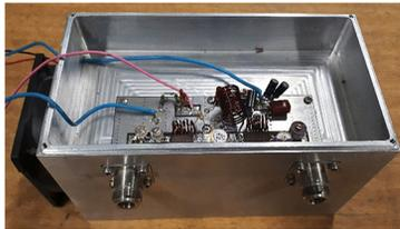
Figure 2: The fabricated 30W pre-amplifier @ 71MHz.
