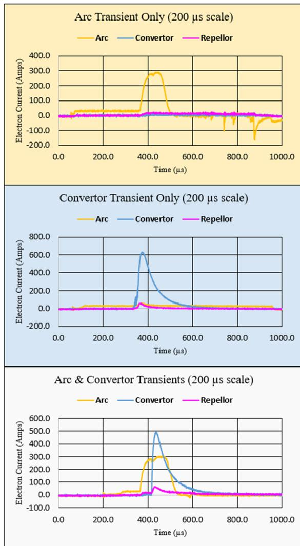
Figure 3: Large transient types observed during controlled test. The top panel shows an Arc only transient. The middle panel shows a Converter only transient. The bottom panel shows combined Arc and Converter transients.
