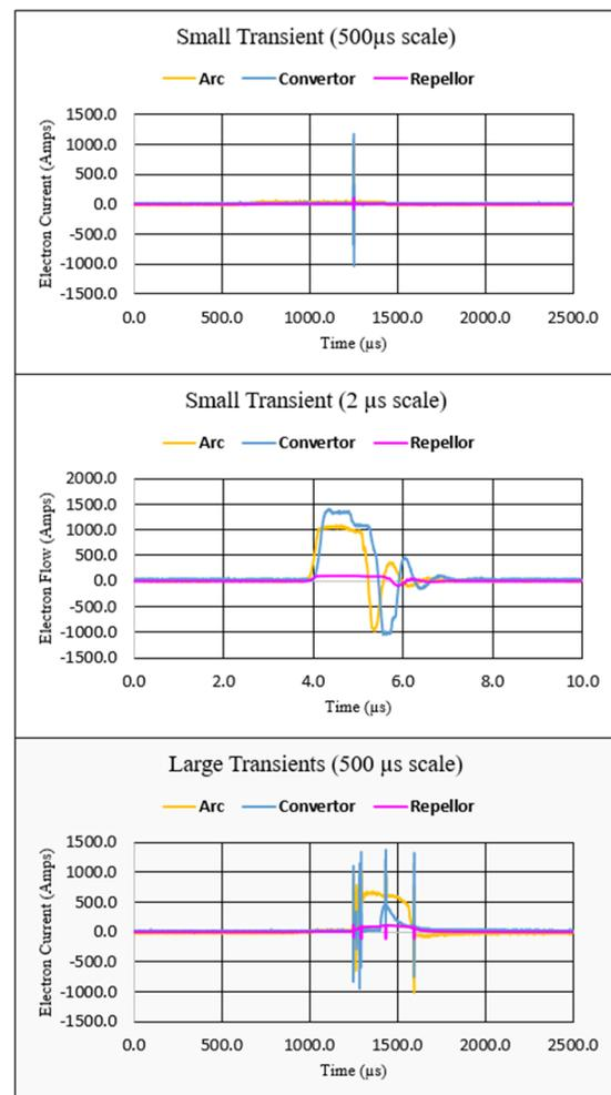
Figure 2: Observed transient in the H- injector operations at LANSCE. The top two panels show small transients (few μs) signals at different scales. The bottom panel shows a large transient (hundreds of μs).
