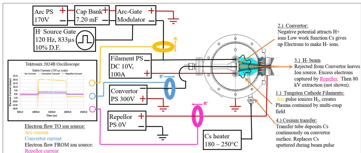
Figure 1: Diagram of H<sup>-</sup> ion source ideal operation.
