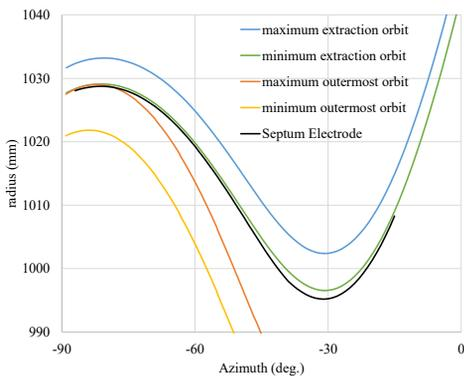
Figure 2: The extraction orbit, the outermost orbit and the position of the septum electrodes in the case of 65 MeV protons in cylindrical coordinates.
