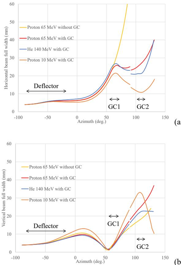
Figure 5: Beam size variation of (a) horizontal and (b) vertical direction at each azimuth with or without Gradient Corrector (GC) in the case of 65 MeV Protons. There are also shown the beam sizes of 140 MeV  ${}^4\text{He}^{2+}$  and 10 MeV protons. Definition of the horizontal direction is the radius of cylindrical coordinates if the azimuth is less than  $90^\circ$  or orthogonal direction to the beamline if the azimuth is more than  $90^\circ$ .
