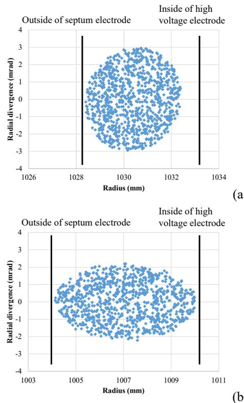
Figure 3: Phase space plot of the proton 65 MeV beam in the deflector. The positions are a) at the entrance and b) at the exit. The positions of the deflector electrodes are also shown.
