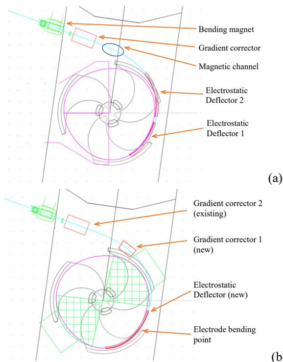
Figure 1: Schematic drawing of a) existing and b) new extraction system of the AVF cyclotron at RCNP.
