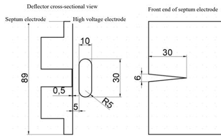
Figure 4: Drawing of the deflector electrodes. All dimensions are in mm. Gap width between septum electrode and high voltage angle is variable from 4 mm to 10 mm.
