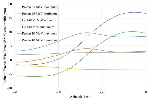
Figure 6: The difference from the central orbit of 65 MeV protons of the maximum or the minimum radius of the orbit of 65 MeV protons, 10 MeV protons and 140 MeV  ${}^4\text{He}^{2+}$ , respectively.
