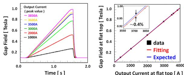
Figure 3: The linearity of the gap field in the NU line to the output current at flat top.
