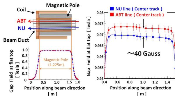
Figure 4: The gap field along the beam direction in the NU and ABT extraction. The error bar of each points is r.m.s. which is approximately 0.15 %.
