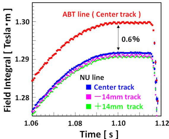
Figure 5: The time dependent BL of the gap field along the NU and ABT line.
