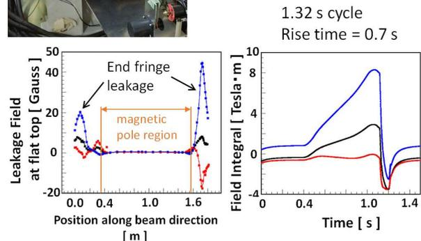
Figure 6: The definition of the tracks for leakage field measurement (Top). The longitudinal distribution along the circulating line (Left). The time dependent BL (Right).
