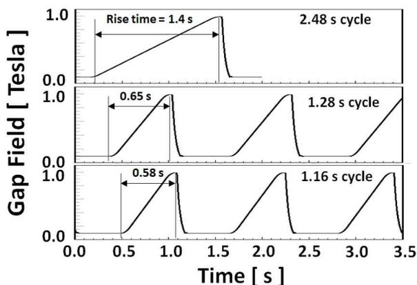
Figure 2: The waveforms of gap field at 2.48 s, 1.28 s and 1.16 s cycle.
