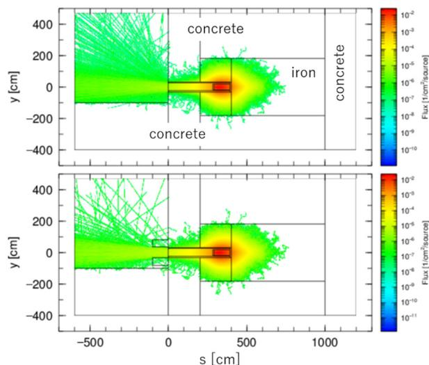
Figure 8: Backscattered neutron flux distributions into the accelerator tunnel.
