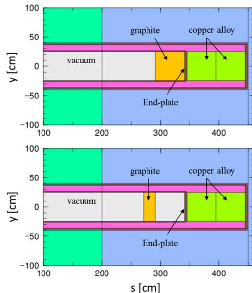
Figure 5: Set-up of graphite moderator.
