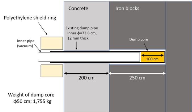
Figure 4: A schematic design of the 30 kW beam dump.
