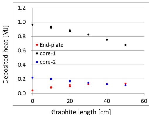
Figure 7: Deposited total heat in dump elements.
