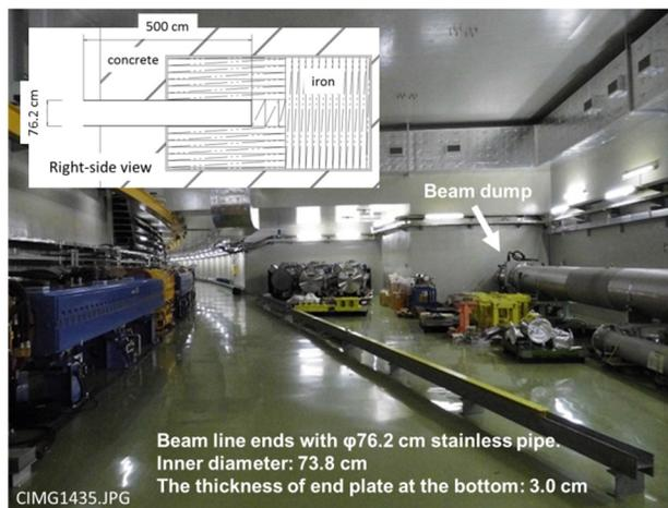
Figure 2: Present beam dump and its structure.
