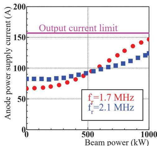
Figure 1: Measurement results for the output current of the anode power supply depending on the beam power. The red circles and blue squares indicate the cavity resonant frequencies of 1.7 MHz and 2.1 MHz, respectively.
