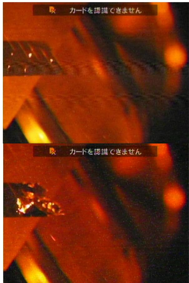
Figure 1: The new HBC foil before (upper) and after 2-month operation (lower).
