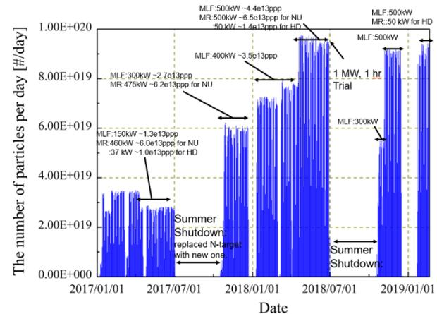
Figure 2: The change in RCS output power with respect to time.
