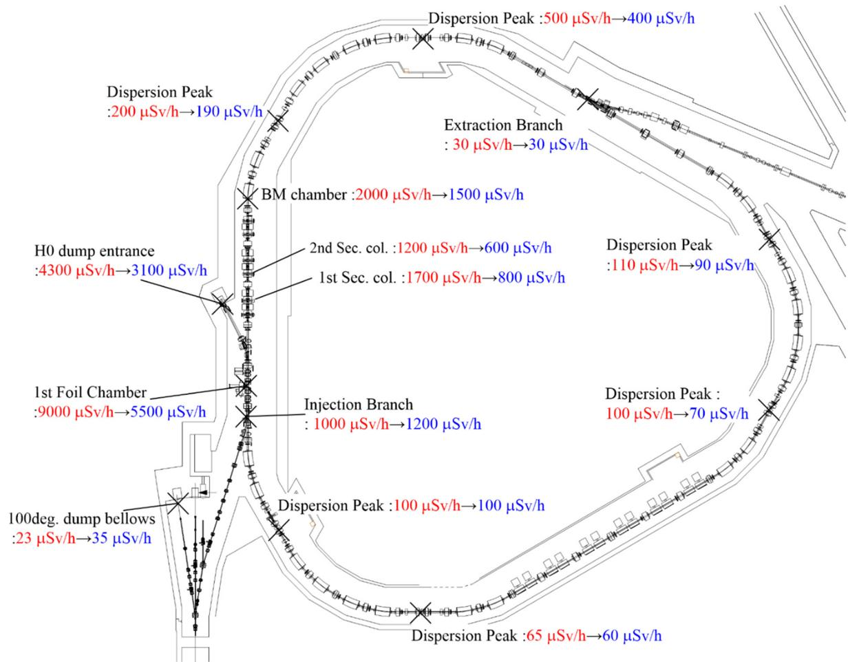
Figure 3: RCS residual dose distribution after 500-kW user operation and 1-MW trial.
